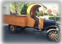
For Sale: 1926 Model TT One-Ton Truck - The carb and water pump have been rebuilt, transmission bands and pedal linkages adjusted Sept '15. New tires fitted. New front fenders, 12v starter, and ahooga horn installed. Starts right up, Muncie drops right into gear without drama, and away you go!
