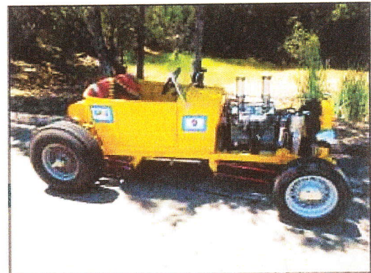
Car #9. Class SP-2. 8.515ET at 070.00 mph. Serr Miller head, '39 trans with Zephyr gears, quick change rear end
