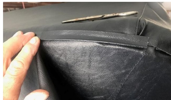
Using a short length of trim as a gauge to make sure final trim out will cover tacks and seams
