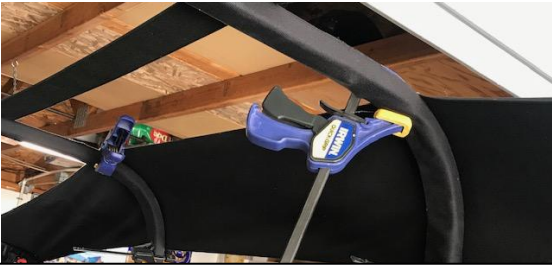
Clamping the pads in place and smoothing out before stitching up.
