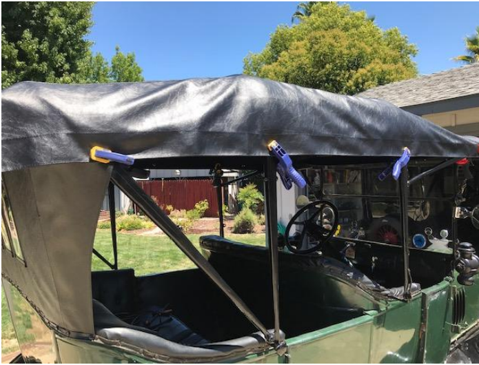
The vinyl top and back before stretching and tacking down.
