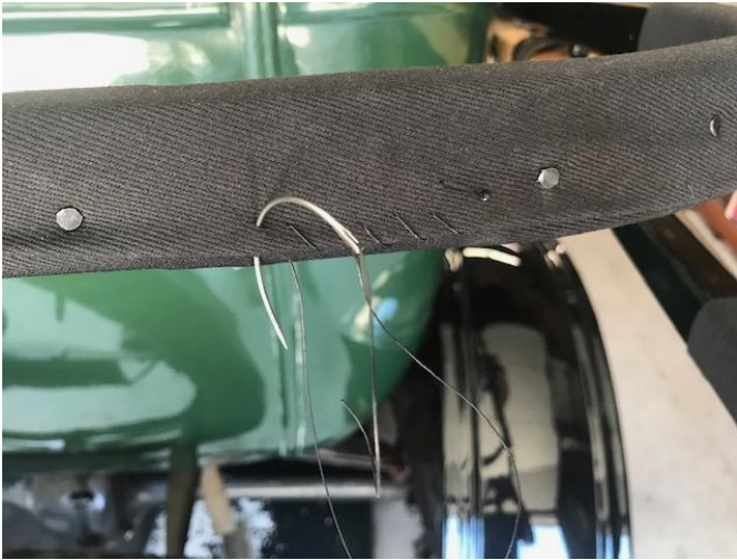
Stitching the cloth bow covering over the metal part of center and rear bows.
