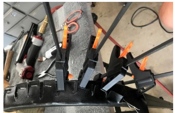
Shaping the vinyl on the curved section of the front bow.
