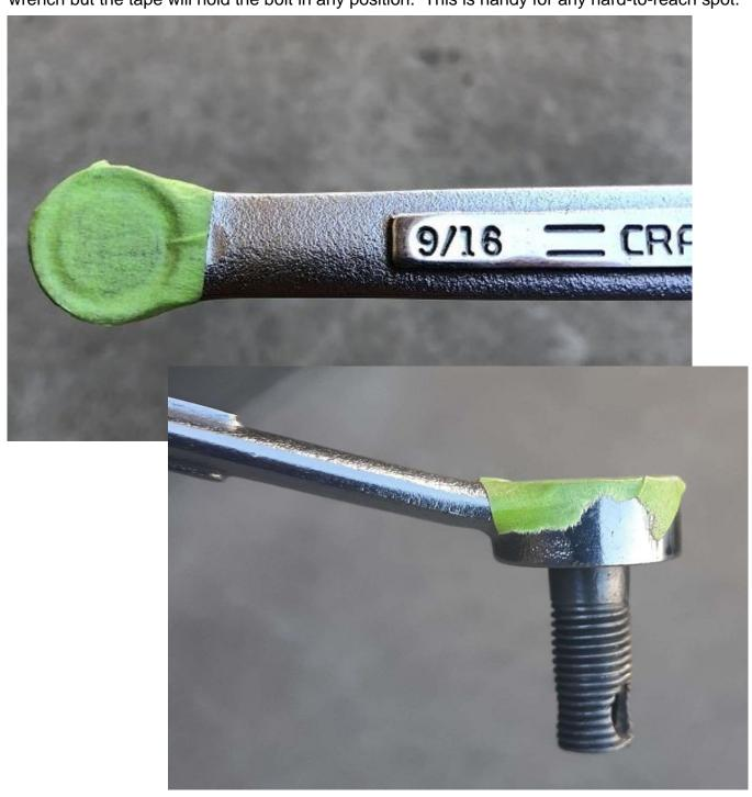
While reading through the Ford Dealer & Service Field, January 1928, I noticed this method to hold the nut. So, even back in the day, mechanics had the same issue and invented a way to make the job easier.
