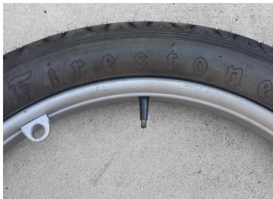
Photo 1 - Valve stem centered on Brand Serial
