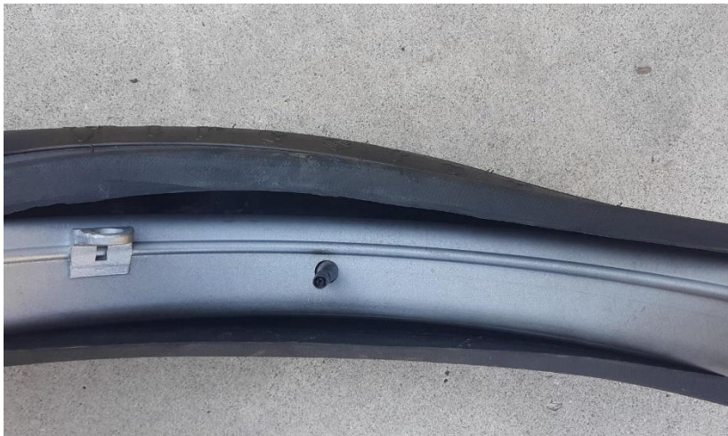
Photo 4 - Press the wheel into tire
