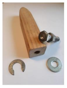
Layout and mark the other end of the block on center. Take a ½ diameter drill bit (I used a Forstner wood bit) and drill a hole from the end down through the center of the block 1 1/2" deep. When you're done, some 80 grit sandpaper will make the edges more rounded and smoother.
